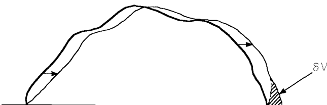
FIG. 5. Deformation of the substrate cross section, which can be treated as a volume increase of \delta V by rescaling.
